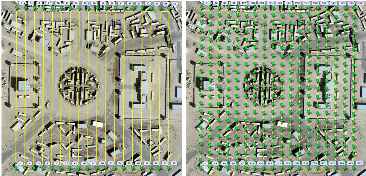
**Figure 1. Striping Flight Pattern**
